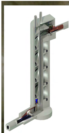
Fig 1 -- Xypex Concentrate and Modified were combined to provide waterproofing and protection for two large shafts at the heart of a new sewage collection and transport system in the Ďáblice district of Prague, Czech Republic. Inset: large drop shaft (shown above) is 118 feet (36 m) tall and 20 ft (6 m) in diameter and features a spiral sewage channel and maintenance staircase.
